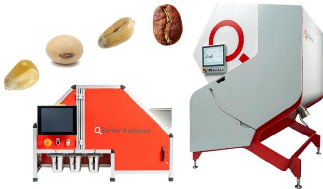
The QSorter® robots are advanced mechatronics devices that have been designed to assess the quality of seeds at the speed of light and sort them accordingly: from 30 to 3'000 seeds per second and one by one. The QSorter® can predict vital seed quality parameters that can be used to predict germination and yield. Sorting for higher germination and higher yield rates enable seed companies and farmers (1) to breed more performing varieties, (2) to increase
