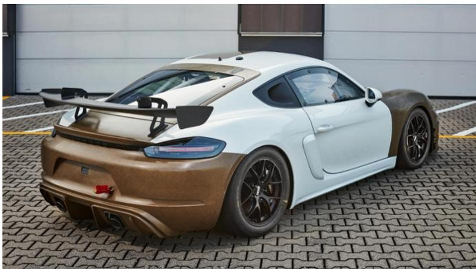
**For the rear wing, layers are impregnated with epoxy resin then baked in an autoclave.**
